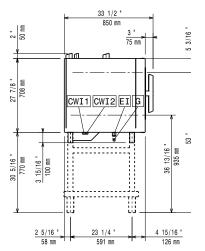
CWII Cold Water inlet 1 CWI2 Cold Water Inlet 2 ΕI Electrical inlet (power)
